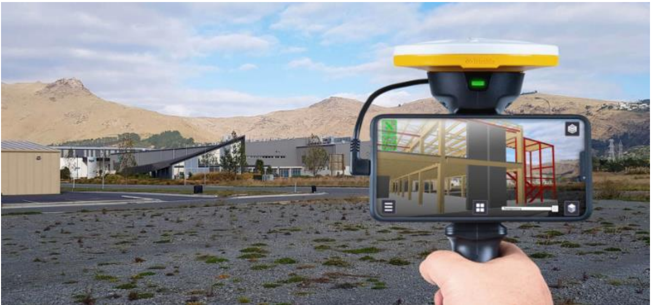
Figure 6: Example of the use of Trimble SiteVision Software
