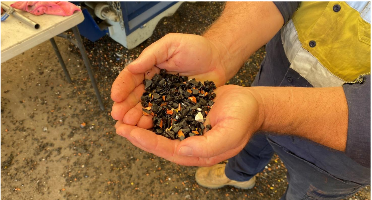
Figure 20 Processed PVC and HDPE plastic pellets from recycled pipes
