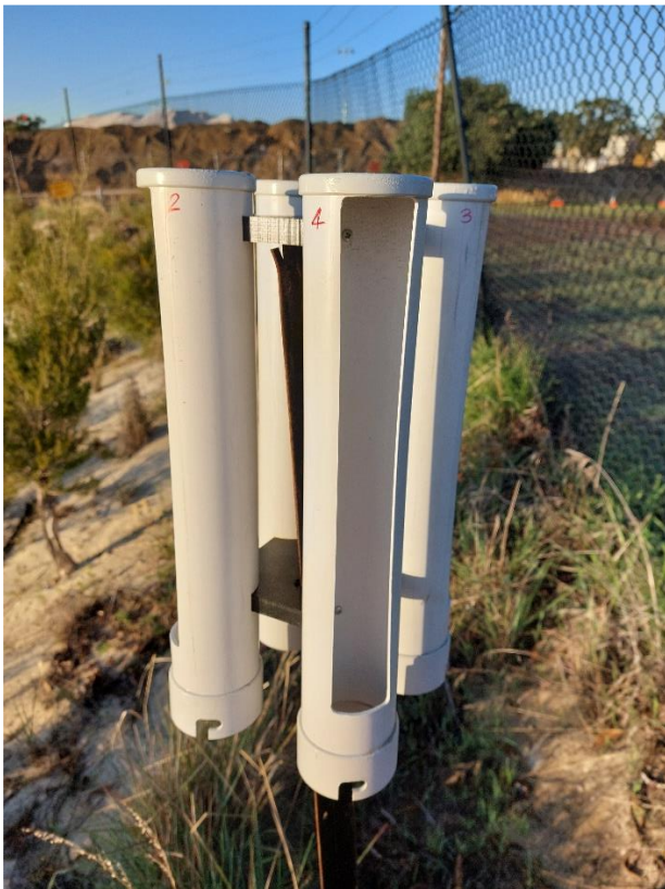
Figure 18 Directional Dust Deposition Gauge in use near Broun Avenue
