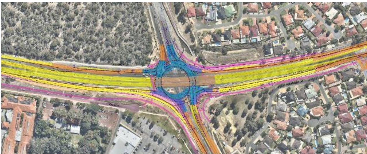
Joondalup Drive & Wanneroo Intersection: Scope- Main Project works which includes Joondalup Drive 4 Span bridge Flyover and modify existing intersection from signalled to Roundabout
